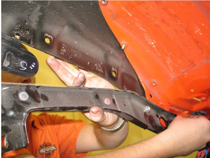
15. Use supplied washers behind shock bolt to replace the thickness of removed struts.
