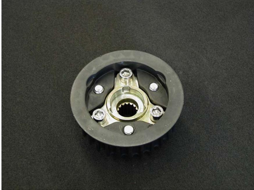
11. Re-install pulley to factory specs with new outer seal. (Don't forget to lube case seal before assembly).
