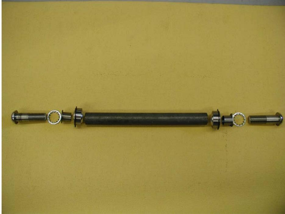
16. Torque shock and pivot bolts to factory specs.
