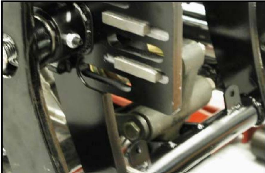
18. Install single sided part of swingarm using supplied bolts and locking tabs (*Do not tighten bolt at this time*).
