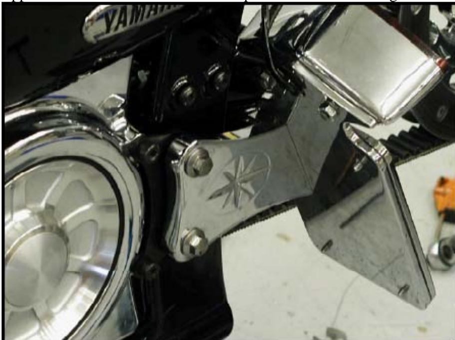
30. Fit and install the rock guard with supplied hardware.
