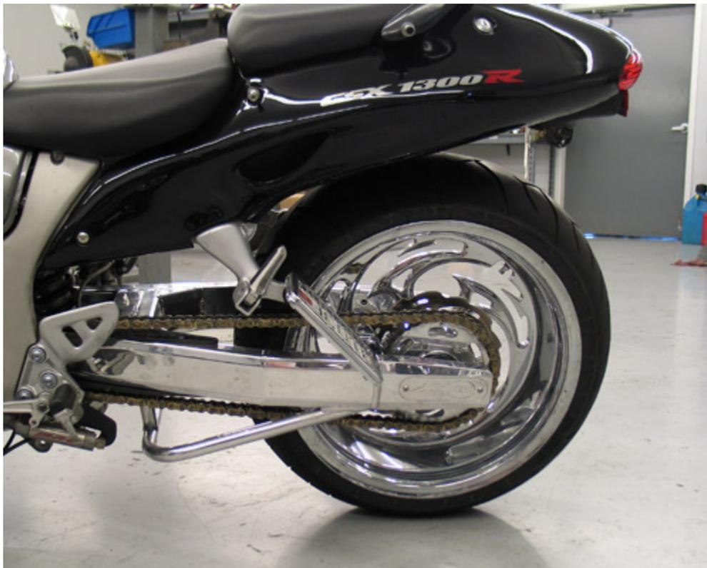
Now that your wheel is installed and the chain is connected, you are ready to reinstall the rear brake assembly. Use the brake fluid type specified on the master cylinder cover. The RC kits have one length brake line for all the kits it has been used for all setups and works great with different routing.
