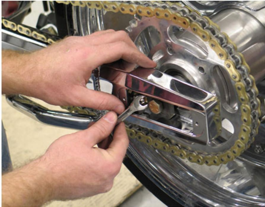
J. Lock down the adjuster bolts and torque the axle bolts to 65-70 ft.lbs.
